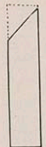
Plane off the edge of the board as shown by dotted lines
