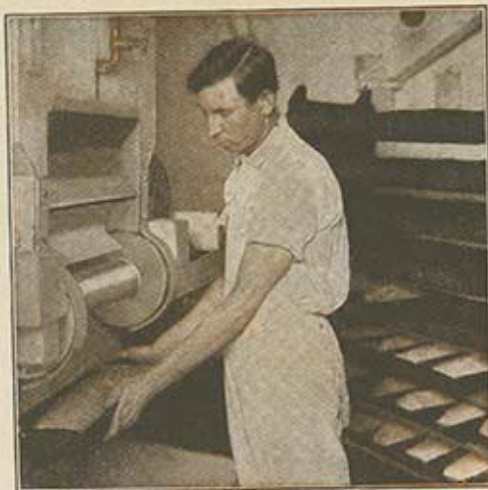
Grape-Nuts Loaf Machine. The dough is cut into exact size and delivered by this device into the baking pan.
